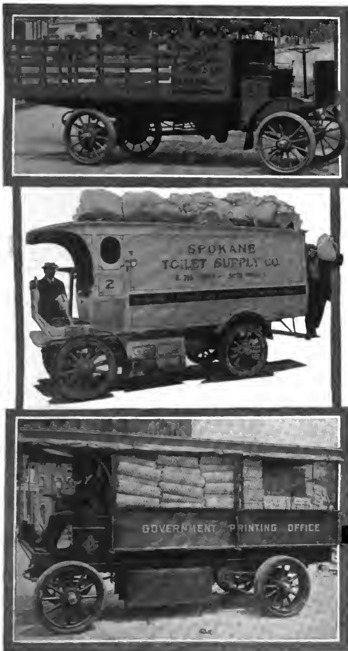
Upper—Ohio 1-ton truck for general contracting work Center—Baker 1-ton vehicle with body suitable for special laundry work Lower—Baker 2-ton truck with body suited to work in government printing service
